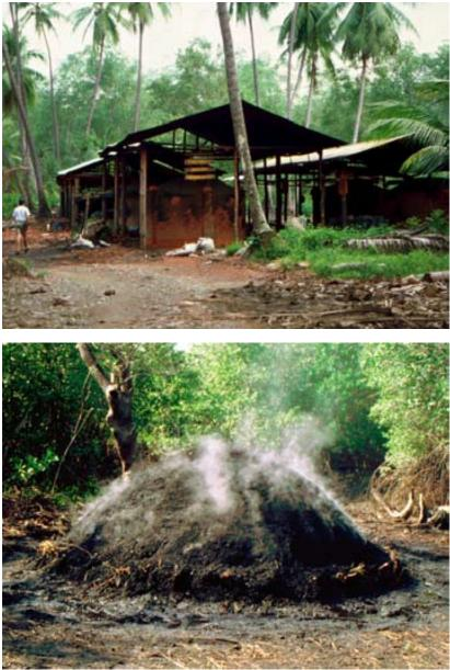
Top: Charcoal treatment plant established with the DANIDA Mangrove Project in Pacific Costa Rica, supported by IUCN and CATIE. Bottom: Typical earthen kiln used to convert stacked red mangrove poles into charcoal for local heating needs, Pacific Panama. PHOTOS: N.C. DUKE
