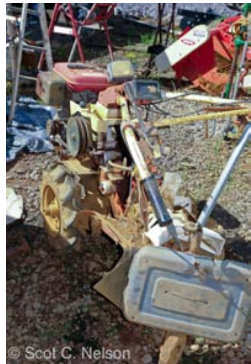
Left: A tractor-drawn and -powered potato harvester is used to dig up sweetpotatoes at larger commercial operations. Right: A mechanized hiller pushed and directed by hand can be used to form mounds of soil within fields before planting sweetpotato vine sections.
