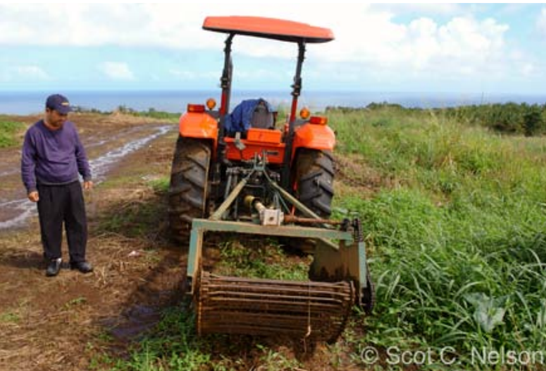
Left: A tractor-drawn and -powered potato harvester is used to dig up sweetpotatoes at larger commercial operations. Right: A mechanized hiller pushed and directed by hand can be used to form mounds of soil within fields before planting sweetpotato vine sections.
