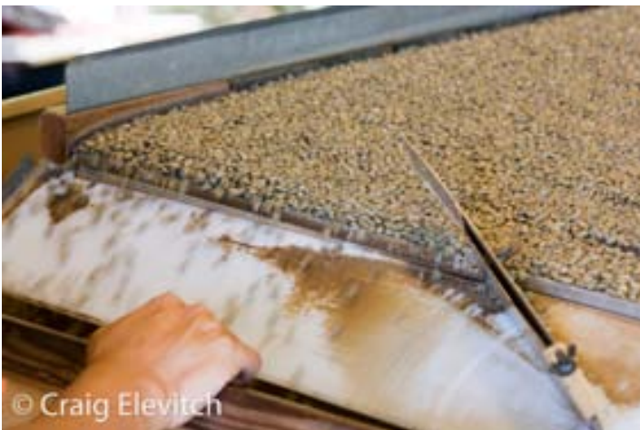
Top left: Covered drying platform with fan to assist in air circulation. Top right: Raking parchment coffee. Middle left: Hand-cranked parchment milling. Middle right: Larger commercial parchment mill. Bottom left: Grading machines such as this table that sorts beans by density are used to remove defective and lower quality beans. Right: Graded and sorted Hawai'i Extra Fancy grade beans.
