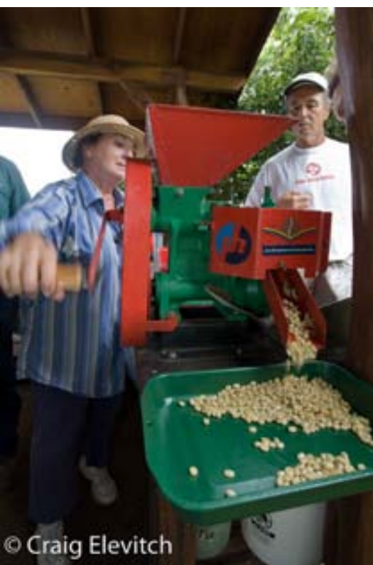
Top left and right: Small mechanized pulpers. Bottom left: A hand cranked pulper can process large amounts of coffee. Bottom middle and right: Pulped coffee beans in a fermentation vat.
